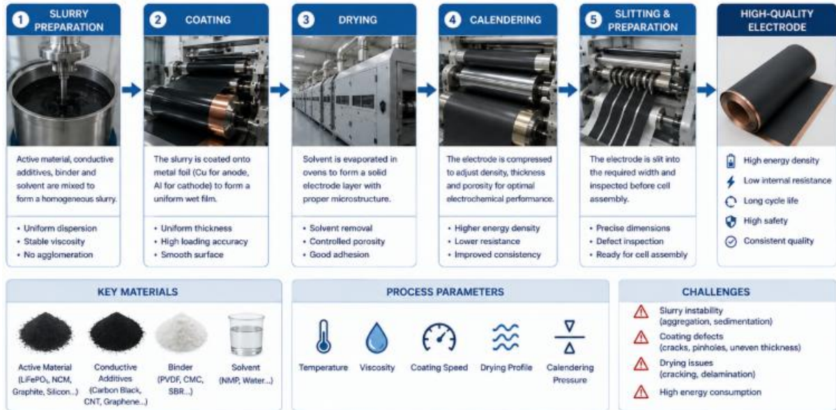
Figure 1. Standart slurry and electrode preparation process [8]
