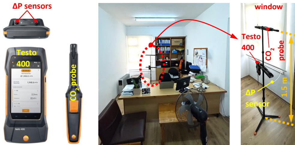
Figure 3. Testo 400 universal indoor air quality instrument and CO 2 measuring probe.
